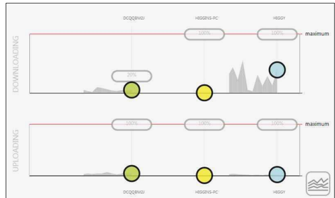
Figure 2: Current view showing real-time bandwidth usage for three home computers in Household D, including an applied download limit of 20% on the computer on the left.
